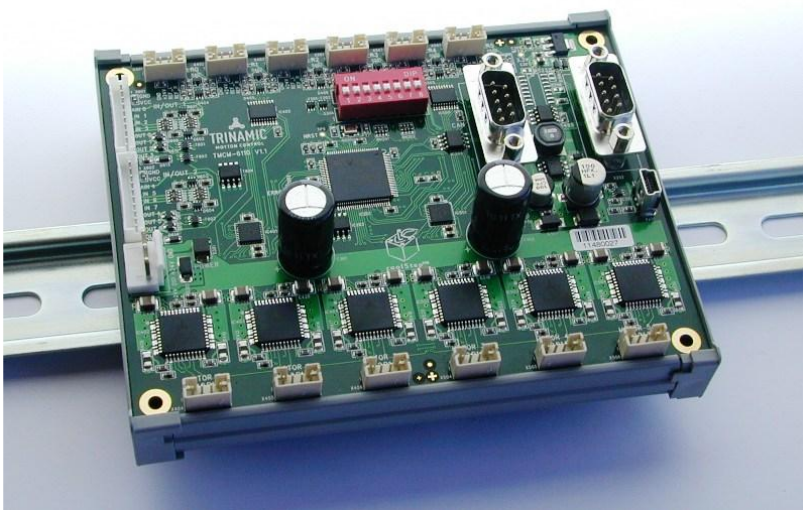
Figure 3.2 DIN rail mounting
